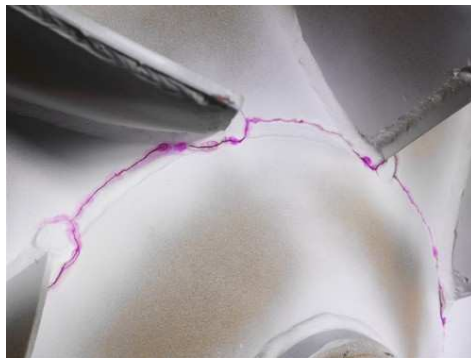
Fig. 3.1 : Dye penetration in the stiffening cone of a turbine.
