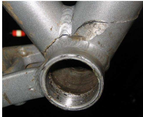
Fig. 1.7 : Crack in a bicycle crank. (Source: internet)
